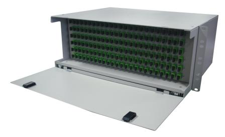
SFO's Fibre Termination Units are used for termination and management of Fibre backbone and equipment cables in Central Office and bulk fibre distribution systems. It serves as the interface between field cables and equipments. Cables may be terminated direct or after splicing. Provision has been made for internal fibre management by cable spooling with minimum bend radius and stackable splice trays. Rack mounted versions are designed for flange mounting on 19 inch racks
