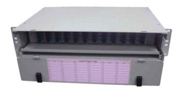
SFO's Fibre Termination Units are used for termination and management of Fibre backbone and equipment cables in Central Office and bulk fibre distribution systems. It serves as the interface between field cables and equipments. Cables may be terminated direct or after splicing. Provision has been made for internal fibre management by cable spooling with minimum bend radius and stackable splice trays. Rack mounted versions are designed for flange mounting on 19 inch racks
