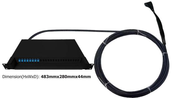
Fiber Termination Units are used for termination and management of Fiber backbone and equipment cables in Central Office and bulk fiber distribution systems. It serves as the interface between field cables and equipment. The 24-fiber cable stub is pre-terminated with SC connectors in the enclosure. Riser-rated and Indoor/Outdoor cable stubs are available in different lengths.
